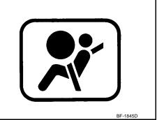
SRS air bag and seat belt pre-tensioner do not operate for approx- Limitately 7 seconds (air bag warning lamp is turning ON) after power switch is turned ON.
