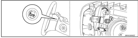
2. Insert a flat-bladed screwdriver (A) into a hole on the left side or the right side of the steering wheel, and place the end of the flat-bladed screwdriver (A) on the torsion spring ①. CAUTION:
