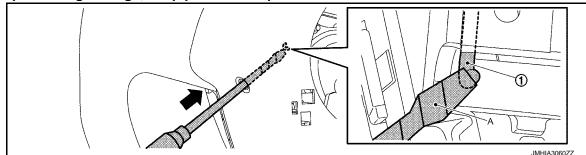
3. Press and hold the driver air bag module on the side where the flat-bladed screwdriver is inserted.
