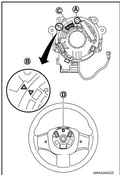
• Fix the driver air bag module harness to the harness fixing hook (A).
