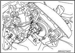
• Press driver air bag module upper (A) until it snaps into place with a clicking sound.
