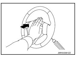
4. Press and disengage the torsion spring ① by using the inserted flat-bladed screwdriver (A).
